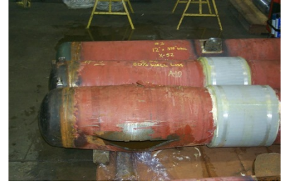
Pipe Body Failure @ 4,260 psi
