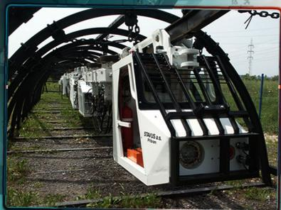
Locomotive IMM 120 TD is a tractive means for transport of train set on monorail suspension lane (profile I 155) aprooved type in horizontal line and also during inclines of elevation or declining about 30°. Locomotive is set together as multipart. It consists of engine part, two separate cabines and additional separate tractive units muttualy connected by linkage.
