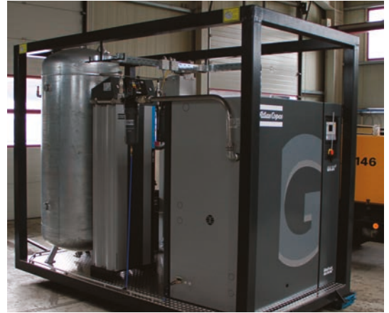
▲ Skid with compressor, desiccant dryer, compressed air tank and filters
